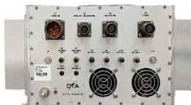
DTA-9590R-4RU 4-Ch. Phase-Coherent Receiver Processing Unit (RPU) with integrated ESM processing. RPU directly outputs Signal Track and Bearing data. (12.62" W x 11.37" H, 6.7" D)
