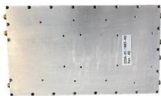
Dual Channel RF Down Converter module (2 used for 4 channels)
