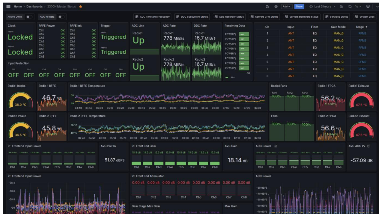
Figure 9: Receive Status monitoring. The dashboard can be easily customized by the user for monitoring specific parameters.
