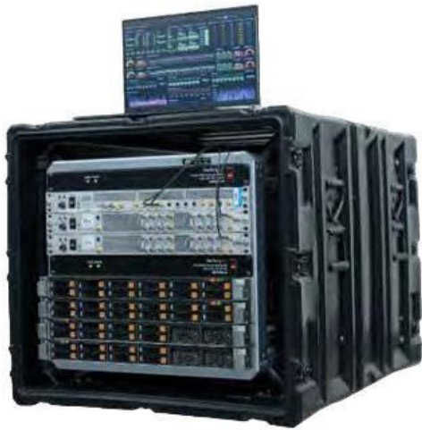
Figure 14: A 64-channel streaming I/Q based OTHR stimulator in a portable carrying case for ease of Rx testing.
