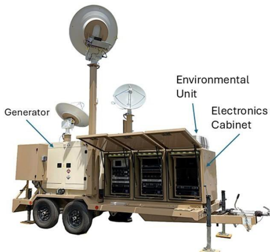
Figure 10(a) shows D-TA's 3-emitter node trailer that includes emitter nodes A, B and C. Fig 10(b) shows a single- node trailer which can include any of the three nodes.
