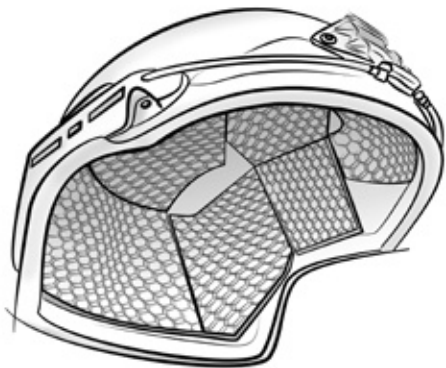
Helmet padding with a micro lattice structure
