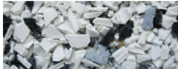
Rozdrobnione profile okienne -10 +0,5 mm PVC - 93,34%, EPDM - 6,66%
