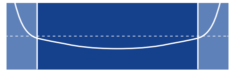
» Thickness profile after MDO without TRIO system
