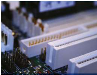
BOARD CONNECTORS VAMPAMID HT 3028 V0 PPA, 30% glass fibre reinforced, UL 94 V0 halogen free
