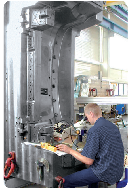
Processing of a 20t injection mold for bumper production.
