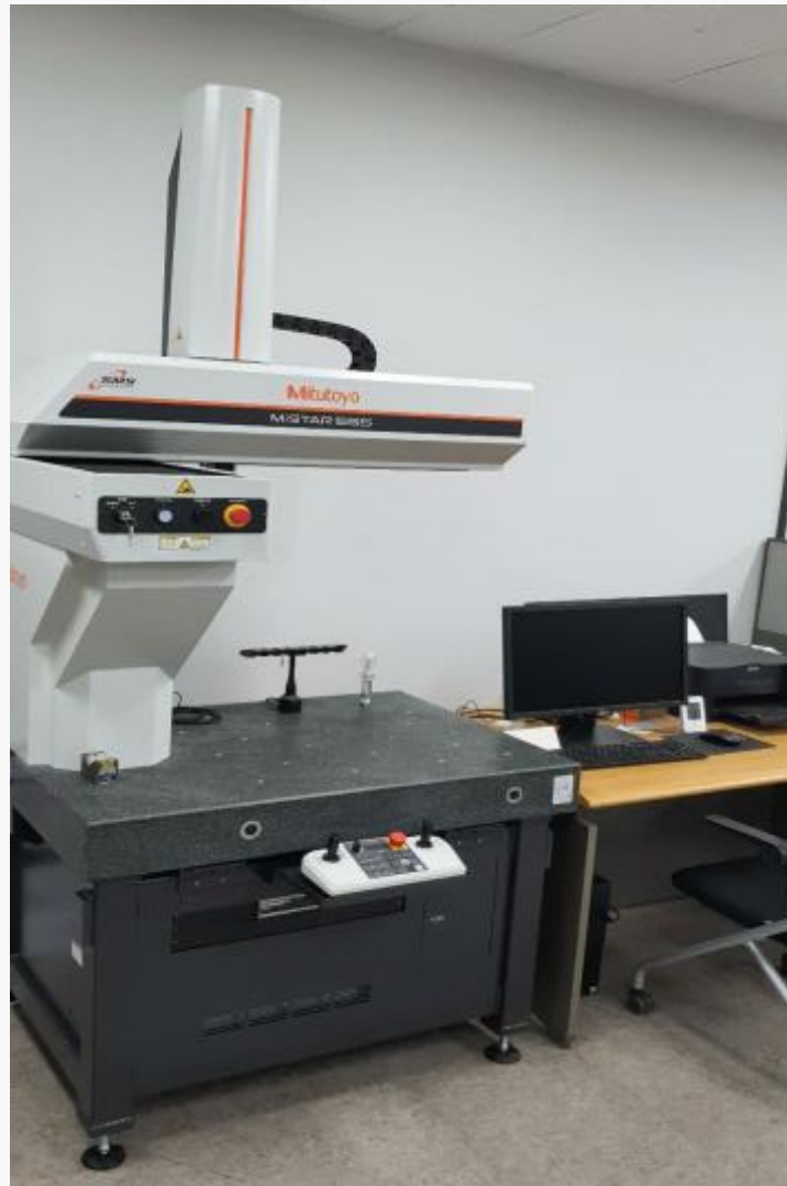
3D Coordinate Measuring Machine (CMM) Mitutoyo MiSTAR 555 (XYZ 570-500-500)
