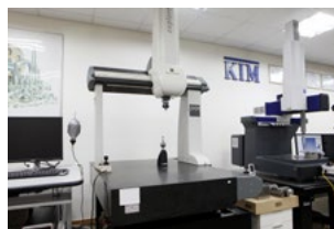
3-Axis CNC Coordinate Measuring Machine Hexagon (USA) Explorer 7105 Spec : 700×900×500
