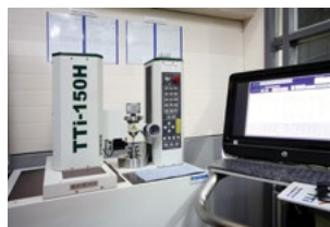
Tokyo Tech (Japan) TTI150H Spec : M (0.3~10) Dia (Φ5~Φ160) Grade (DIN2)
