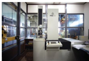
Klingelnberg (Switzerland) PNC65 Spec : M (15) Dia (650) Grade (DIN2)
