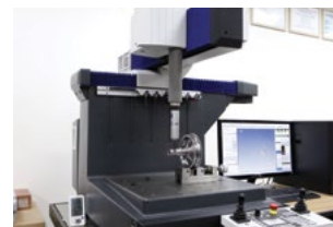
ZEISS 3D Measuring Device Measuring Ranges: X=500 mm, Y=500 mm, Z=500 mm
