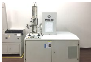
Klingelnberg (Switzerland) PNC30 Spec : M (0.3~15) Dia (Φ5~300mm) Grade (DIN2)
