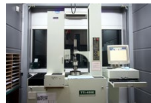
Tokyo Tech (Japan) TTI450E Spec : M (0.3~10) Dia (Φ5~Φ450) Grade (DIN2)
