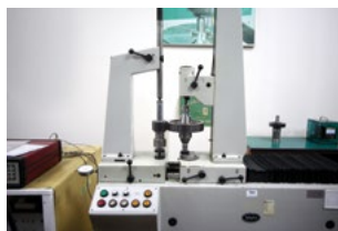
Mahr (Germany) 898D Center Dis. (25~600mm) Grade (DIN2)
