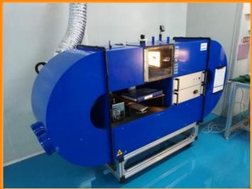
This tunnel was imported from UK. The test tunnel feature exceptional airflow stability and test flexibility, it can simulate the human living environment to test product performance.
