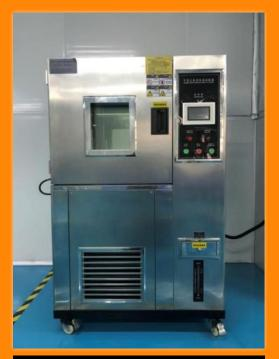
Programmable Constant Temperature and Humidity Test Chamber
