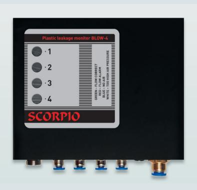
BLOW-4 is an independent four-channel controller detecting raw material leakages in mould hot runner installation space. It is constructed by our company team in response to customers' problems with raw material leakage in small hot runner moulds. Thanks to thorough study of the problem, we created a reliable device with absolute efficiency of leaks detection. It allows to control (via potential-free contacts) the alarm signal and stop the machine operating in case of leakage detection.
