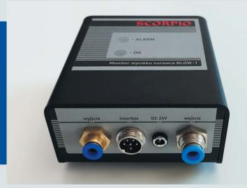
The device, that allows you to minimize failure costs and machine downtime caused by raw material leakage from injection nozzle
