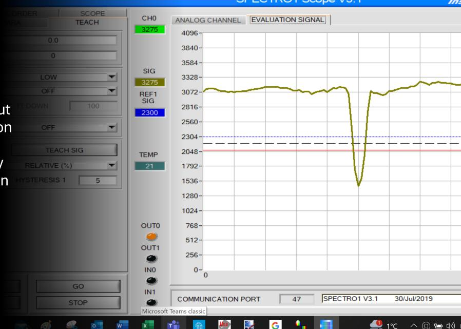
Three laser analog sensors with a laser light curtain of 3mm x 0.5mm each are required to detect the defects over the entire circumference of a 4mm diameter hose.
