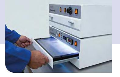
The cliché plate carries the print image. Teca-Print supplies all types of plates suitable for pad printing: plastic plates, steel plates, steel plates 05 and ceramic plates. Each type of plate can be sub-divided into further subcategories.
