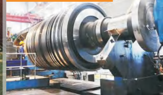
Nuclear Power Rotor Automatic Welding
