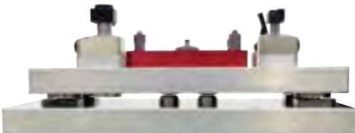
③ Locating + clamping of the fixture completed
