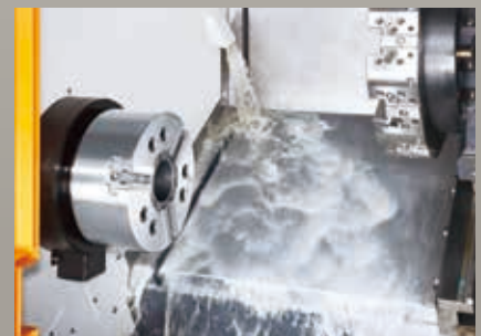
Coolant flush onto covers
