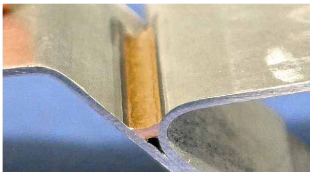
Triple spot brazing creates virtually perfect seams
