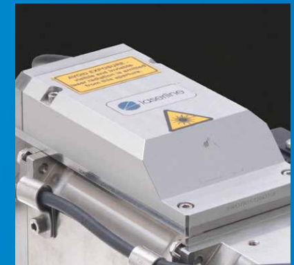
The electronic optics monitoring system controls the parameters throughout the entire process. This ensures that laser power and optics are always operated in the optimum range.
