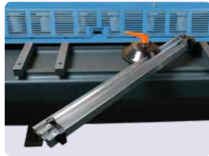
Protractor for angle shearing.
