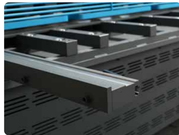
Squaring arms and front support arms with or without scale, T-slots and tilting stop. Lengths from 1000 up to 3000mm.
