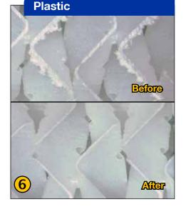
The FLADDER® deburring and finishing principles fundamentally different from which rub tightly against the part, closely those of traditional methods.
