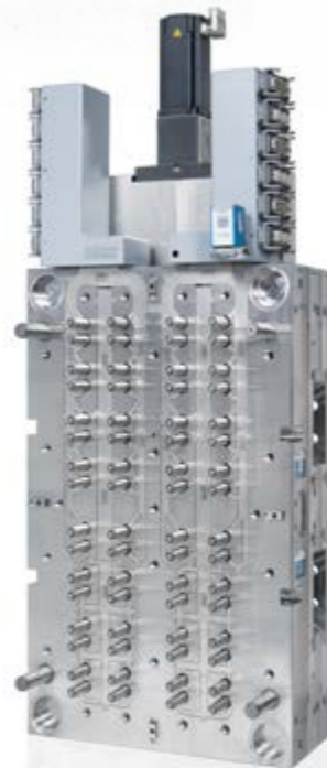
männer Hot Half 64-drop with electrical plate actuation (e-plate)
