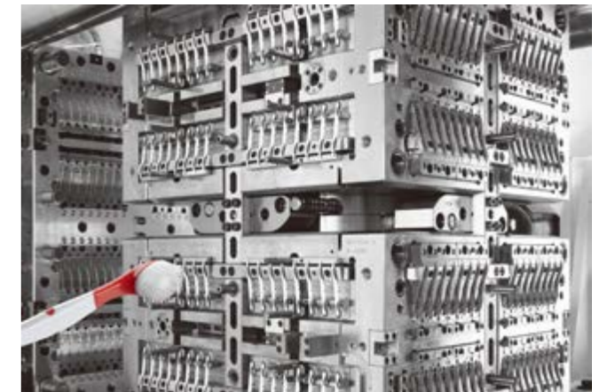
FOBOHA STACK-TURNING molds With the FOBOHA stack-turning technology, parts are processed within the turning system at different levels. So it is possible to inject parts on both levels in the same production step and eject the finished parts at the available station.
