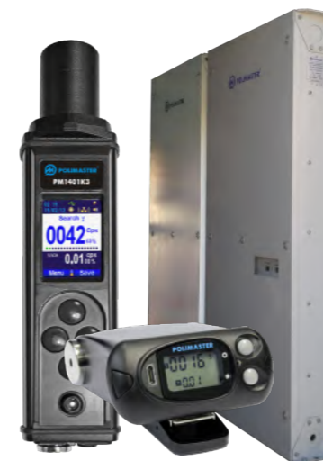
MDS is equipped with Radiation Portal Monitors for prompt detection, and additionally with PM1703 PRD and PM1401K-3 HHRM for localization and identification of detected sources
