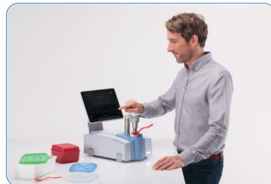
Fig. 1: Measurement of a plastic spoon using the ALPHA II with ATR measurement interface.
