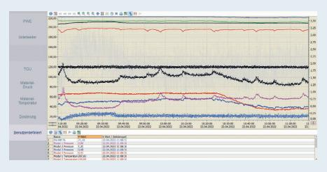
During the process, every step and every variation of each process parameter is recorded so that the data can be correlated to bigger machine sizes.
