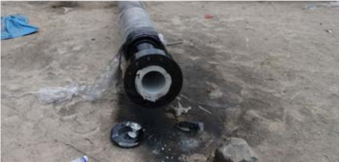
► Internal coating of pipelines for high-temperature crude oil (80 °C) – available only in English language
