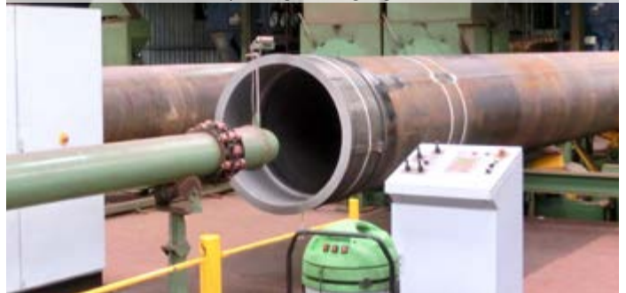
► Internal coating of cooling water intake risers for extensive FLNG-Project in Australia – available only in English language
