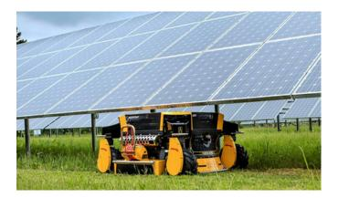
Spider mowers are gentle on terrain and eliminate erosion on slopes. Moreover, its lightweight aluminum alloy design allows for low fuel consumption, resulting in low emissions. Machines can also be equipped with biodegradable fluids that are often required when maintaining ecologically sensitive areas.
