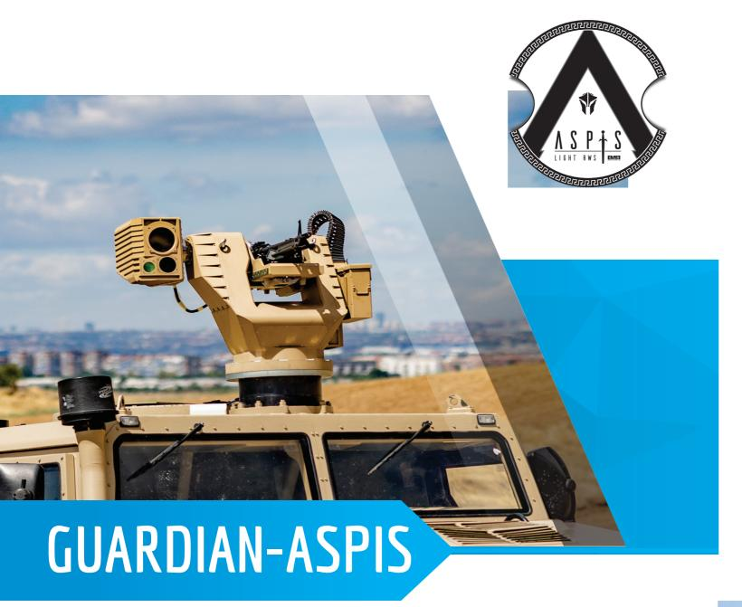
**GUARDIAN-ASPIS** is the lightest remote weapon station on the market. With under 100kg, this 2-axis gyro-stabilized system is capable to operate both during day and night operations.
