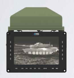
**DVE Alert Multi S** provides enhanced situational awareness in adverse weather, nighttime, and in battlefield operations. Its compact flexible design makes it a drop-in replacement for legacy day periscope and night vision systems. Drivers and crew are provided with enhanced high-resolution visible and thermal images of surroundings.
