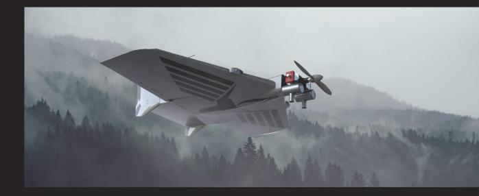
UAV "Hunter Killer" (HaKi-20) is an unmanned aerial vehicle created by Ukrainian engineers, which is designed to neutralize the enemy at a two-way distance of at least 1000 km with the ability to carry a payload weight of up to 15 kg.
