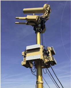
AUDS is a patent pending system that detects, tracks and neutralises UAS engaged in hostile airborne surveillance and defeats, malicious activity. The AUDS system combines electronic scanning radar detection and classification, Electro-Optic tracking and the Claw directional inhibition system operating across 5 frequency bands (GNSS, 433 MHz ISM, 915 MHz ISM, 2.4 GHz and 5.8 GHz ISM/WiFi).
