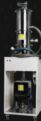
The unit is used for collection of non-reactive metal powder from the build chamber of 3D printer.
