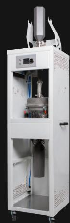
The unit is used for sieving, mixing and homogenizing of metal powder for reuse.
