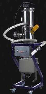
The unit is used for collection of non-reactive metal powder from the build chamber of 3D printer.
