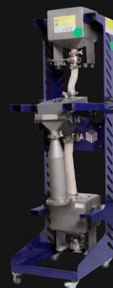
The unit is used for sieving, mixing and homogenizing of metal powder for reuse.
