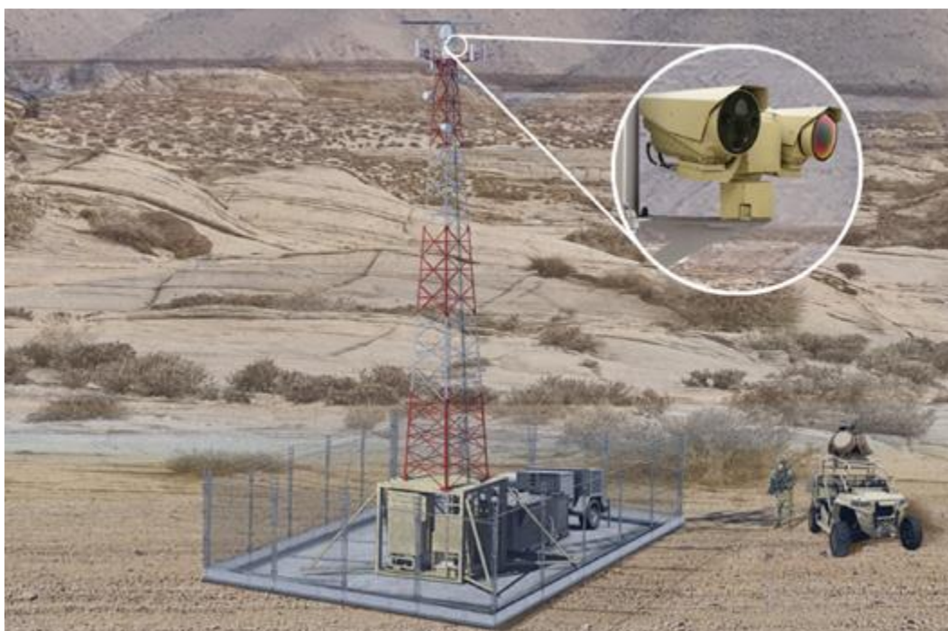
Figure 1 – Multiple sensor outstations (radar, AIS, EO)
