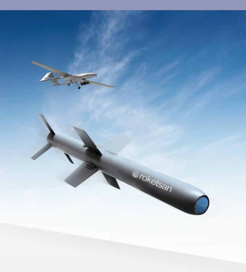
MAM-C lightweight Smart Micro Munition has been developed for unmanned aerial vehicles [UAV] and light attack aircraft, and for air-to-ground missions where weight is a critical factor.
