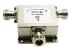
Type N Circulator from 300MHz to 10 GHz
