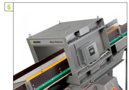
6 Metal detector DLS and DLS-R Separable tunnel metal detectors of type DLS and DLS-R can be installed in (existing) conveyor belts and guarantee highest detection accuracy throughout the whole aperture area. DLS metal detectors typically are used for the protection of cutting mills and shredders.
