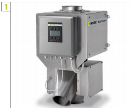
1 RAPID VARIO-FS Metal Separator Compact free-fall separation system. Metal contaminants are rejected via the rejection flap of the "Quick Flap System" without disrupting the material flow.
