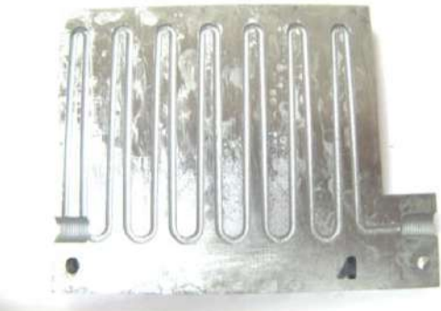
1.2709, with AnoxPro coating, approx. 10 \mu\text{m} layer thickness
