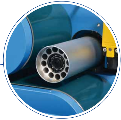
Sensor roller for monitoring the synchronous speed between the upper and lower belt
