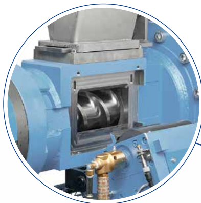
Extruder with open feed roll chute
