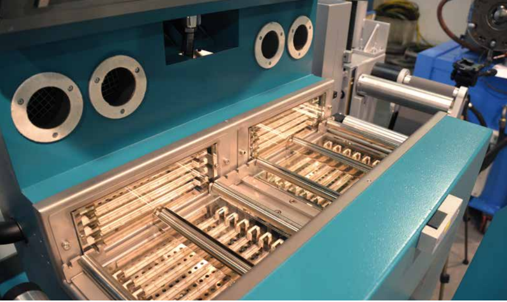
Horizontal air-cooled infrared pre-shock for 360° application.
