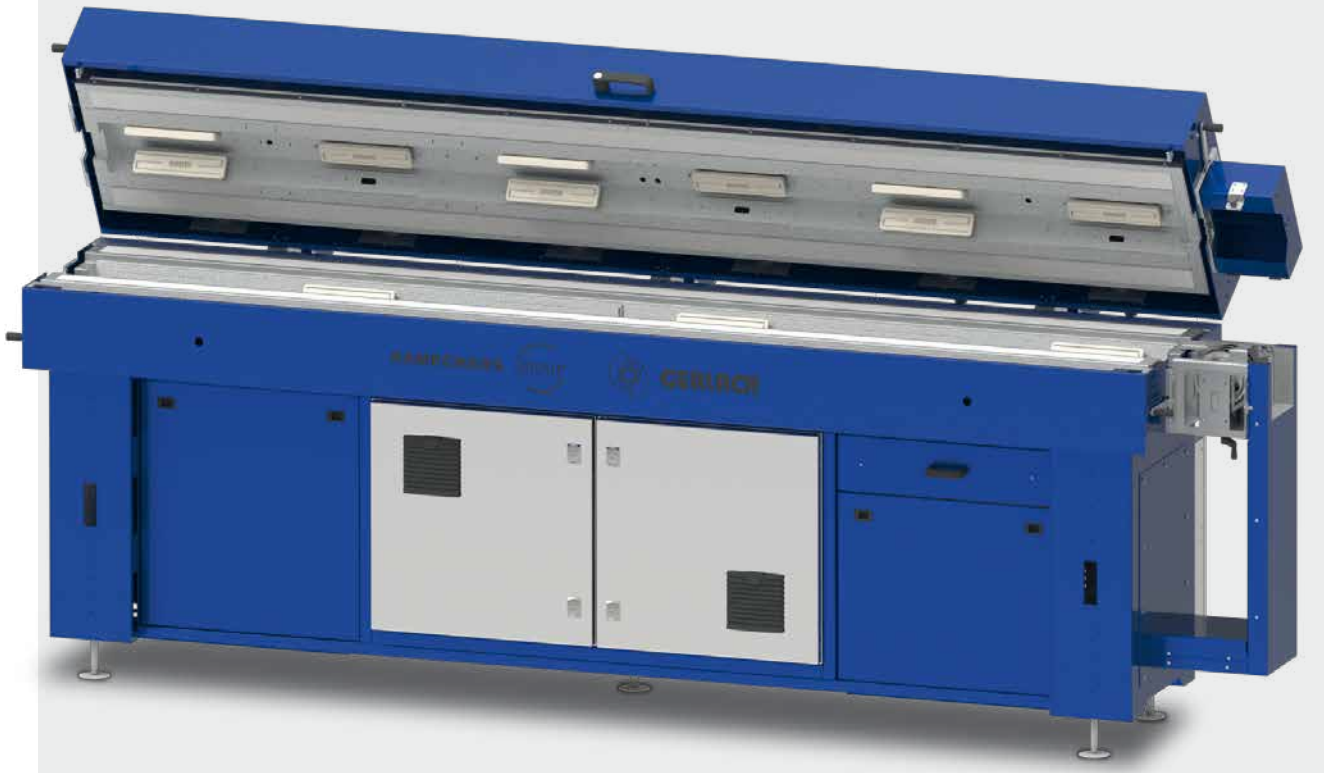
HEX 330 cable machine with infrared emitters
