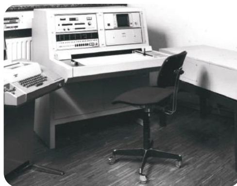
Early IFS Series with 'Genzel' interferometer set many standards in research FT-IR.
