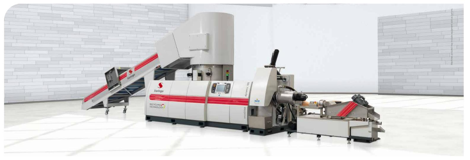
State-of-the-art recycling technology with extended functionalities such as SMART feeder and dynamic automation package. Designed for processing film, fibres, thermoplastic in-house production scrap and washed post-consumer waste from materials such as PE, PP, PET, PES, PA, PLA, PS, PPS as well as foamed products. The most efficient solution for hygroscopic and wet materials.
