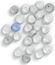
First analysis and identification of contaminated pellets
