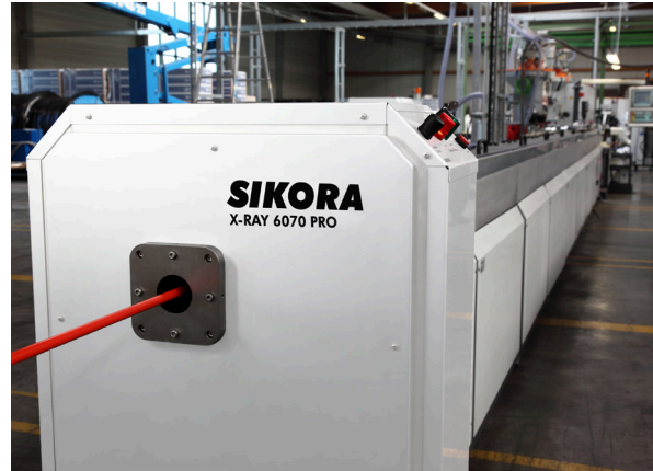
X-RAY 6070 PRO integrated in a production line
