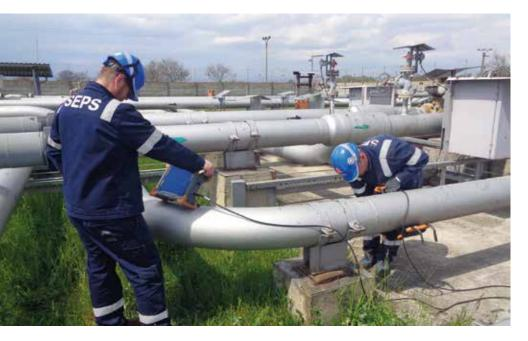
The probe performs the so-called volumetric measurement, which is then converted to the average residual wall thickness.
