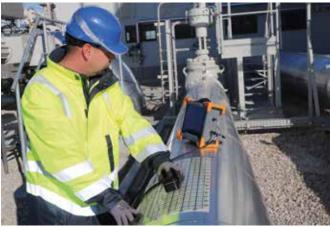
The measured thickness values are relative, representing the wall thickness change (loss of material) at the examined structure, calculated using the reference material thickness from the place where the probe was calibrated.
