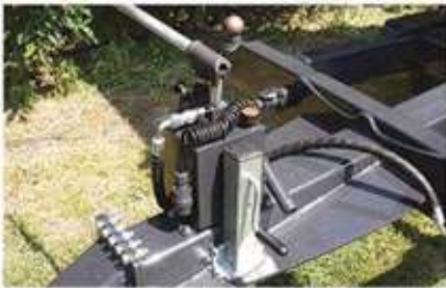
■ Manual pump for supported leg or box tipping (selected models)
