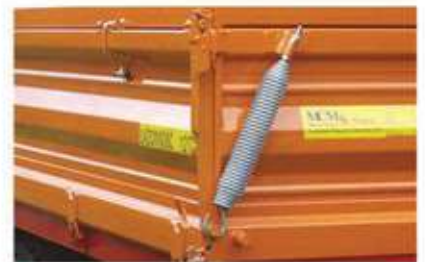
■ Side walls springs (only available when walls made of closed profiles)
