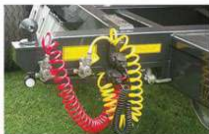
■ One circuit hydraulic or air brake system or two circuit air brake system
