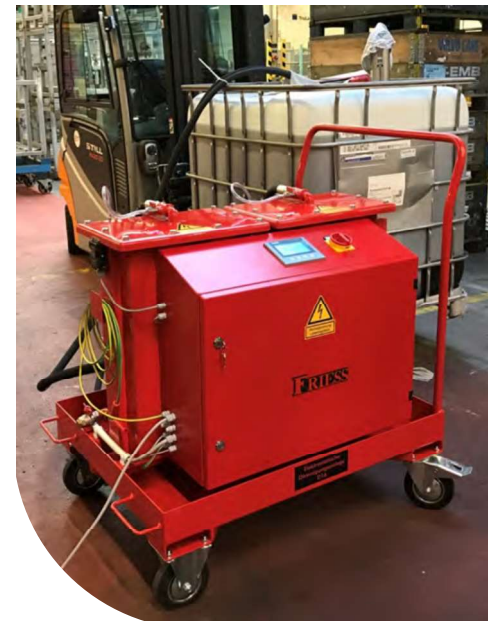
Electrostatic oil cleaner D16 in operation
