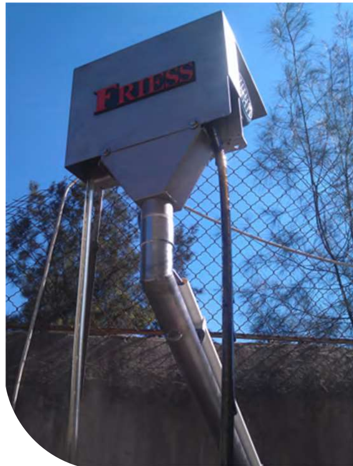
Oil skimmer in operation. Oil is picked up on one side, scraped off in the skimmer and the clean tube comes down the other side.
