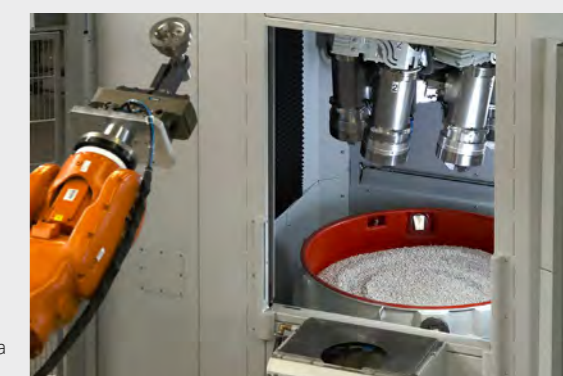
Robot attaching a work piece to a workstation in the drag finisher
