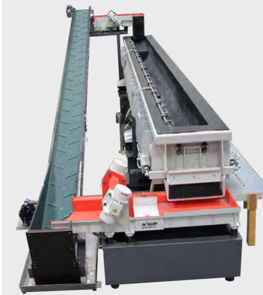
Tub vibrator with external media classification
