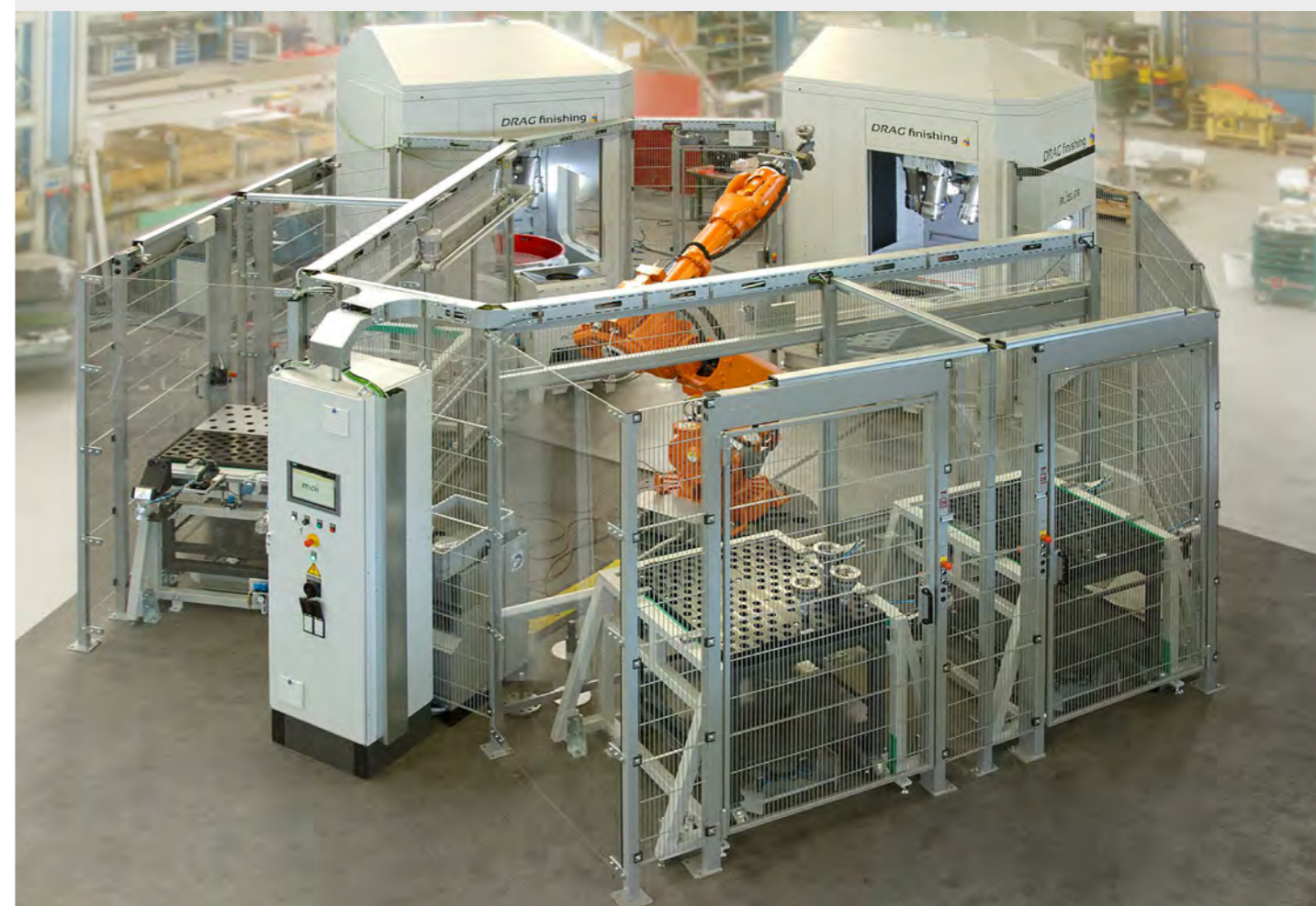
2 drag finishers with robotic loading/unloading of the work pieces
