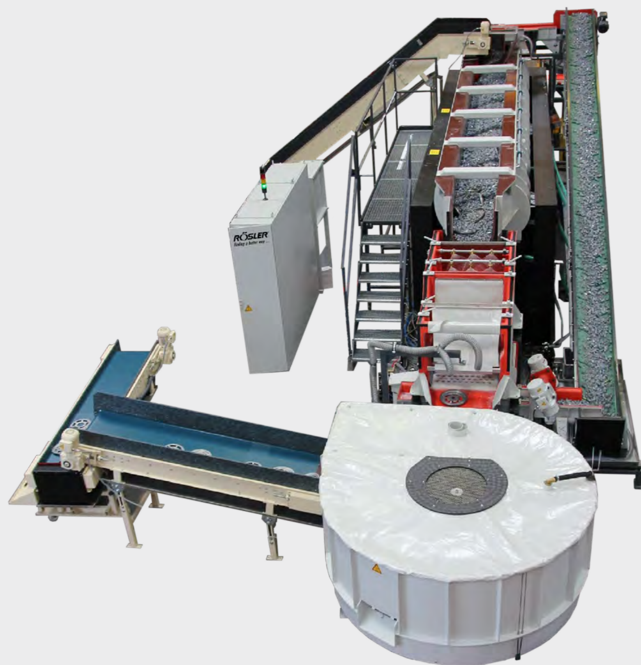
Linear continuous flow vibrator linked with loading belt conveyor, rotary dryer and various transport belt conveyors.
